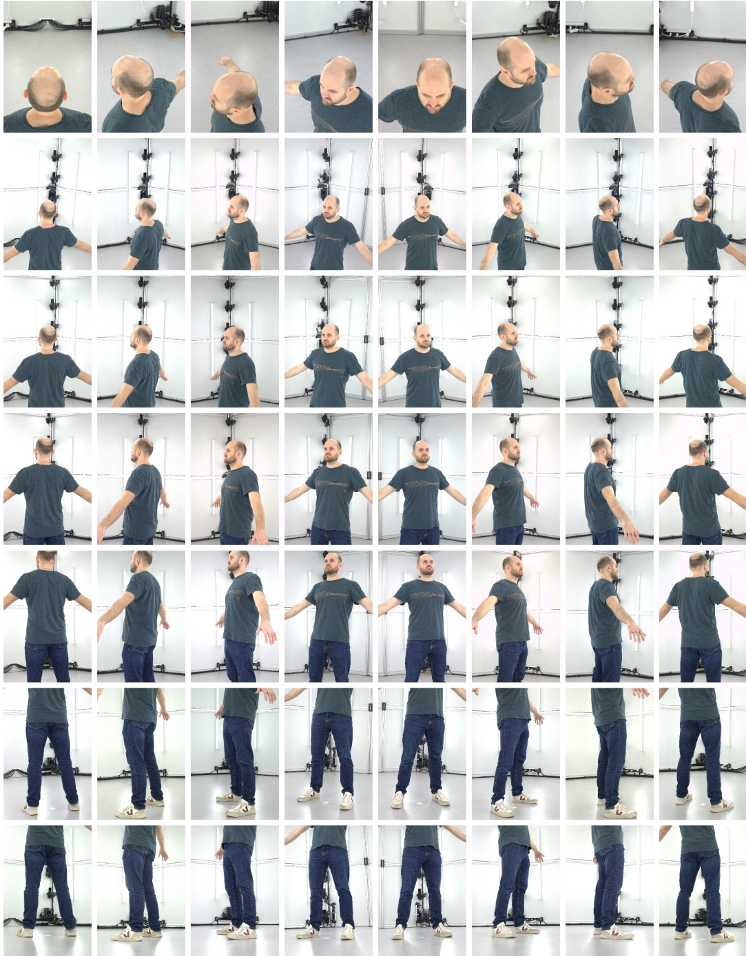
Figure 2.2: A set of images created by our photogrammetry rig. 56 cameras are evenly distributed to capture the scanned subject from all angles. These images are passed to a commercial photogrammetry software in the next processing step of our virtual human creation pipeline.
