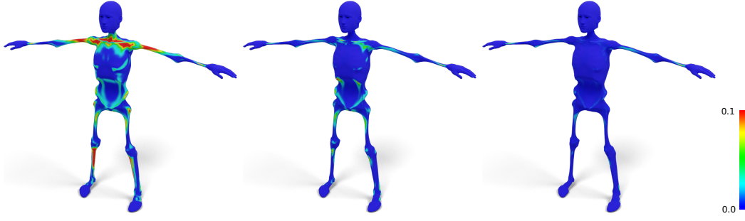
Figure 6.5: Standard non-rigid registration from skin to skeleton (left) results in a bad tangential alignment of corresponding triangles, causing sheared prisms, which we visualize by color-coding the alignment error (6.4). Using fixed correspondences reduces this error (center). Shifting closest point correspondences with bad alignment reduces the error even further (right).
