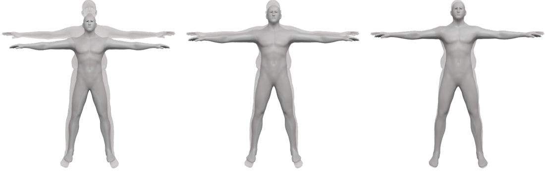
Figure 6.7: Scaling the template (opaque) to match the scan (semi-transparent): The preprocessing aligns the scan with the template and puts it into the same pose (left). Body height and limb lengths of the template are then adjusted by a global uniform scaling (center), followed by local scaling for limbs and spine (right).
