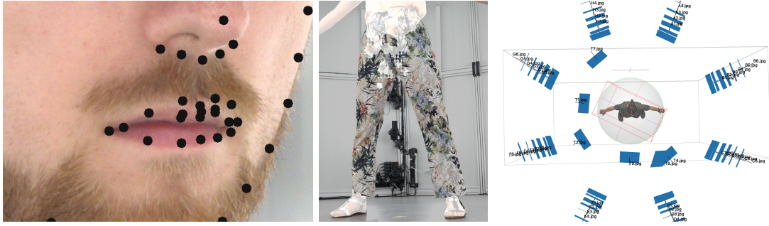
Figure 2.9: Failure cases of the presented virtual human reconstruction pipeline. The facial feature detection can fail to correctly detect the mouth region. Note that the left mouth and the lip center line is not detected correctly (left). The image segmentation can fail to accurately segment the scanned subject. Here, the pants with a floral pattern are erroneously masked from the input image (center). Lastly, the camera calibration performed by Agisoft Metashape can misalign some of the top cameras. Three of the eight top cameras are not aligned correctly in the depicted example (right).
