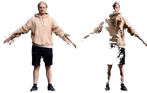
Figure 1: Point cloud from all images (left) and sub-scan capturing the left part of the subject. The full point cloud exhibits noticeable motion artifacts in both arms.
