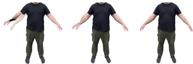
Figure 9: Comparison of avatar renderings in scan pose over input images (transparent) using 0 (left), 2 (middle) and 5 (right) sub-scans. An increasing number of sub-scans improves pose alignment and geometric accuracy (right arm).
