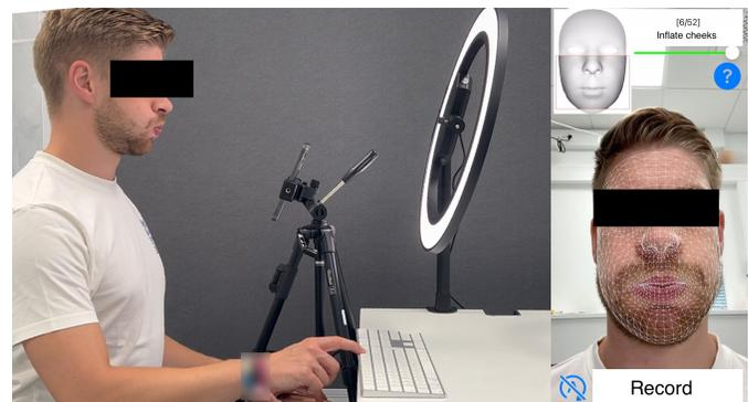
Fig. 5: *Facial Expression Capture.* (Left) Capture rig with tripod-mounted phone and ring light, (right) user interface.
