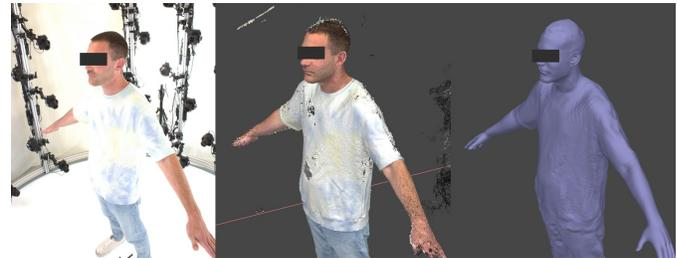
Fig. 4: *Body Reconstruction.* (Left) Images from 94 DLSR cameras are transformed into (center) dense point cloud, then (right) template mesh model is fit into pointcloud.
