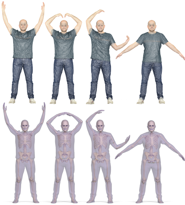
Figure 12: The results of fitting our model to different scan poses (top row). We first unpose the scan by fitting our human skin surface template. The skeleton inference is then performed in the trained A-pose. Finally, we employ linear blending skinning to repose the results back to the observed scan pose (bottom row). Note that the fingers of the second pose are not faithfully reproduced by the pose estimation of the employed template fitting technique.
