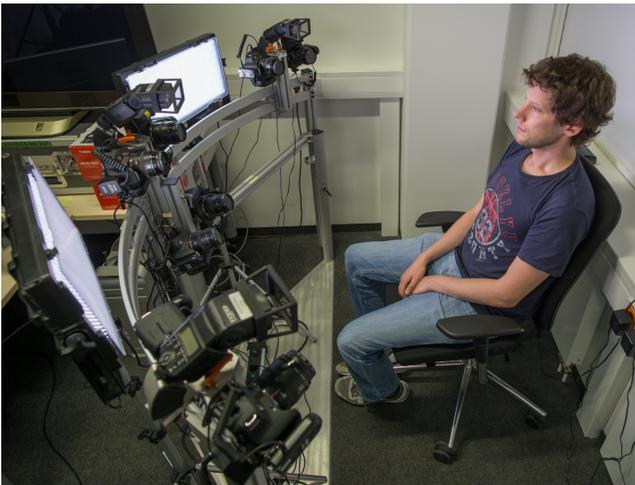
**Figure 10: The developed photogrammetry rig used to specifically scan the faces to achieve higher texture resolution.**
