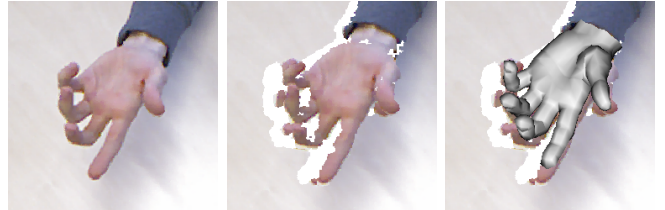
Fig. 1. The user’s hand posture is estimated in real-time by fitting a 3D hand model to the Kinect point cloud using inverse kinematics.
