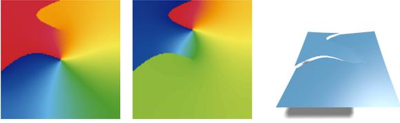
**Figure 9:** Multiple progressive cuts within an element: The harmonic enrichment textures  $H^i(\xi)$  for each of the cuts (left, center), and the resulting simulation behavior (right).
