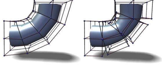
**Figure 2:** Comparison of embedding techniques. Stitching the discontinuous simulation mesh, followed by barycentric interpolation, leads to  $C^0$  artifacts (left). In contrast, our smooth MLS-based embedding yields a considerably higher surface quality (right).
