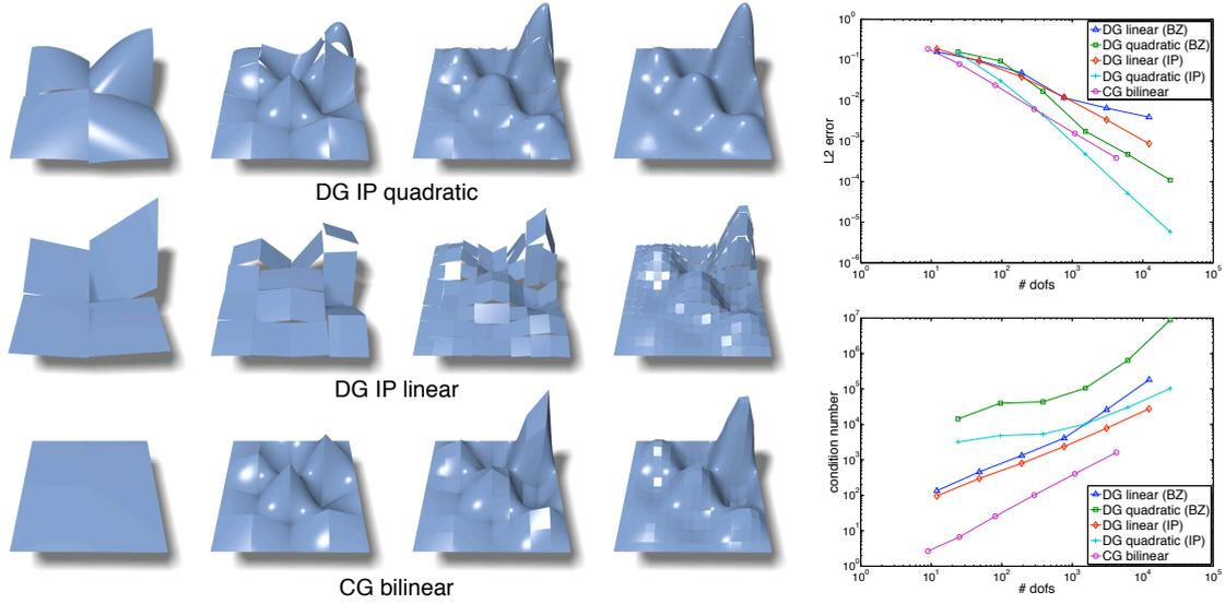
**Figure 4:** Solution of the Poisson equation  $-\Delta u = f$  on a regular quadrilateral grid of resolutions  $2^2$ ,  $4^2$ ,  $8^2$ , and  $16^2$ , using CG FEM and DG FEM. The plots compare the  $L^2$  errors  $\|\Delta u + f\|$  and the condition numbers of the stiffness matrix  $K$  for the BZ and IP method using linear and quadratic basis functions, and also include bilinear CG FEM as a reference.
