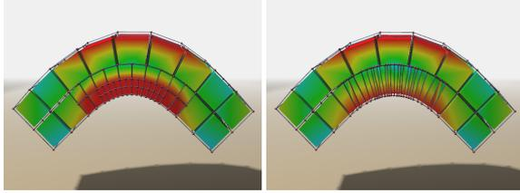
**Figure 6:** A bar (36 hex-elements) is dynamically refined during bending. 1-to-8 subdivision results in 274 elements (left), whereas 1-to-2 refinement yields 77 elements (right).
