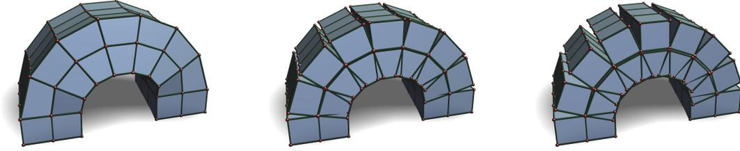
**Figure 1:** Comparison of CG FEM (left), DG FEM (center), and the elastically coupled rigid cells of PriMo [BPGK06] (right). The DG method conceptually spans the whole space from CG to PriMo, since for sufficiently large penalties  $\eta$  it approximates the CG results, and for an extremely stiff material and lower penalty  $\eta$  it reproduces the rigid cells of PriMo.
