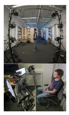
Figure 2: Our custom-built full-body scanner (left) and face scanner (right) are both based on multi-view stereo and consist of 40 and 8 DSLR cameras, respectively.
