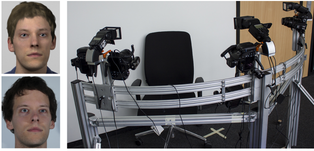
Figure 2: Our face scanning setup (right) and comparison between photographs and virtual reconstructions of our actor (left).
