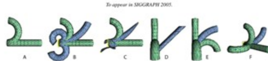
Figure 5: Using MESHK to pose a bar. (A) Two example poses superimposed on top of each other. (B) The left cap of the unbent bar is constrained to stay in place while a single vertex on the right side is manipulated. Three edits using our nonlinear feature space are shown. Note that MESHK generalizes beyond the two examples and can create arbitrary bends in the plane. (C) In contrast, the linear feature space interpolates and generalizes poorly. (D) In this top-down view, moving the constrained vertex perpendicular to the bend causes a shear since no examples were provided in this direction. (E)-(F) Providing one additional example in the perpendicular direction allows MESHK to generalize to bends in that direction as well as in the space in between.
