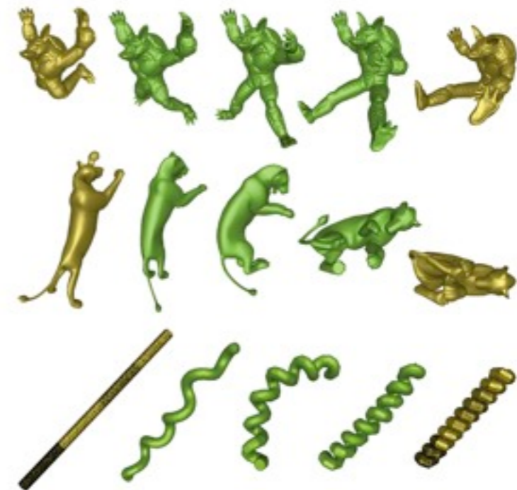
Figure 6: Interpolation between two input meshes (leftmost and rightmost columns). The interpolated poses (in green) are shown for parameter values of t = 0.25 , t = 0.5 , t = 0.75 .
